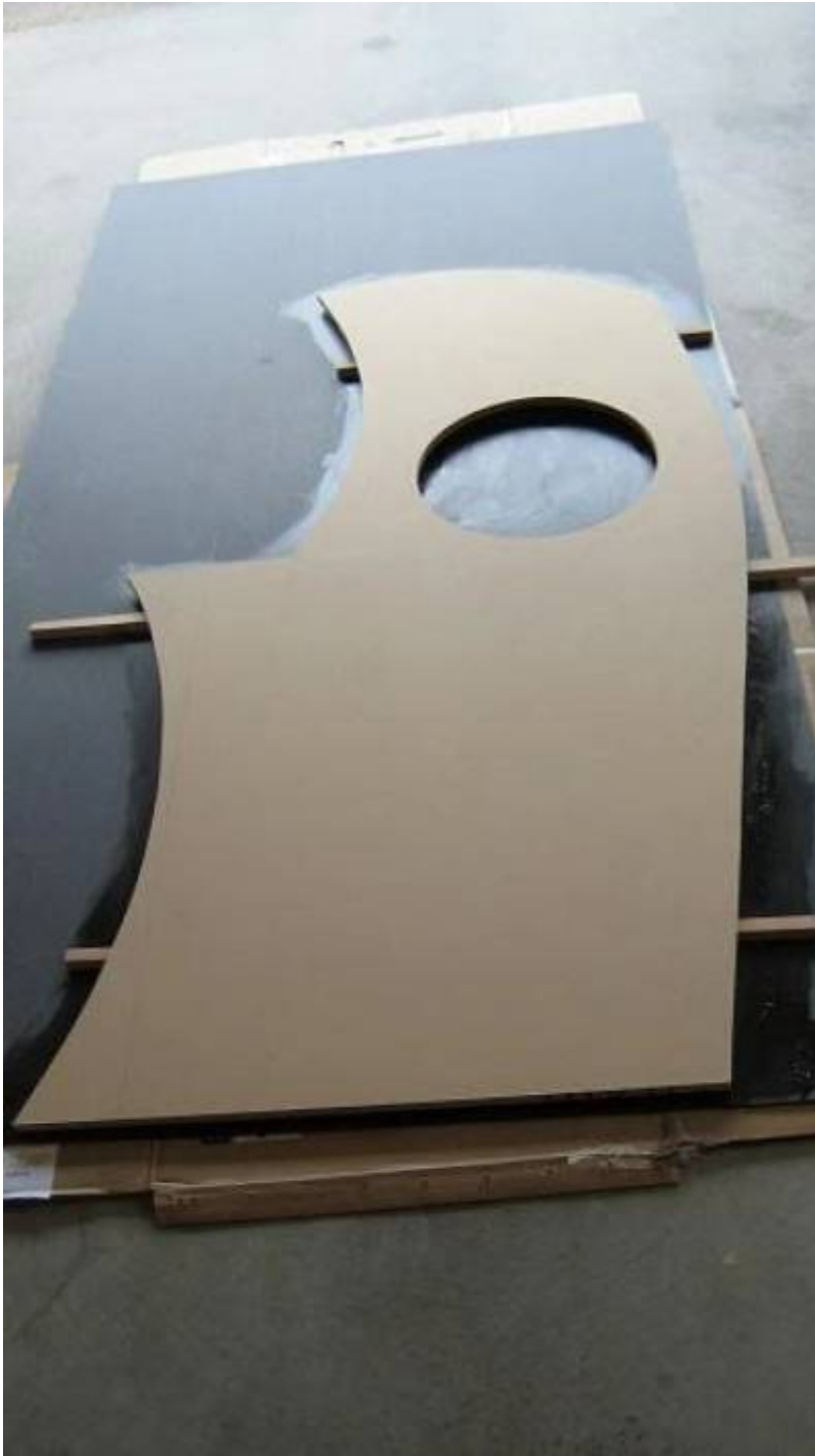
Here is the outside of side 1 fully laminated before and after side hole was trimmed:
