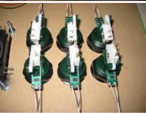
Here is the wiring complete for the LED Wiz...the mini rats nest on the top left will be organized further...getting tired! You can see to the right of the nest a euro terminal block that is feeding the 5 volts for the Lighting. The 5v runs to a hacked molex plug which will hang beneath the CP.
