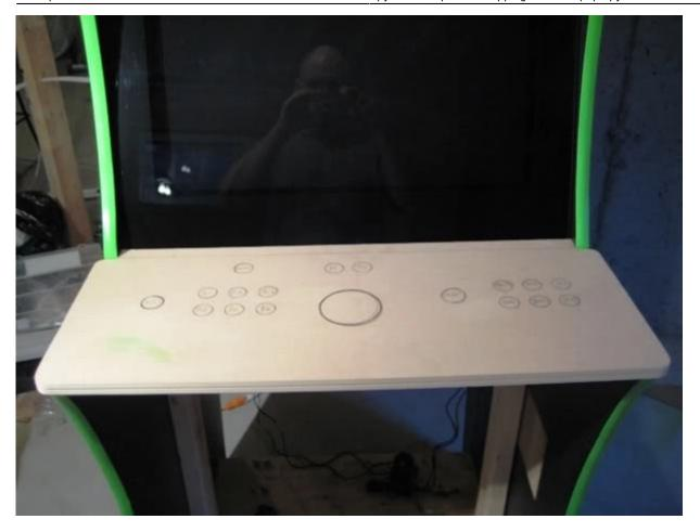
First few tests of the curved piece worked fine. To create my own bendable MDF I have been cutting slots to within 3/16" down, spaced 3/4" apart on 3/4" MDF. I will then put glue in the slots and mold the curve. Ill document this step in closer detail.
