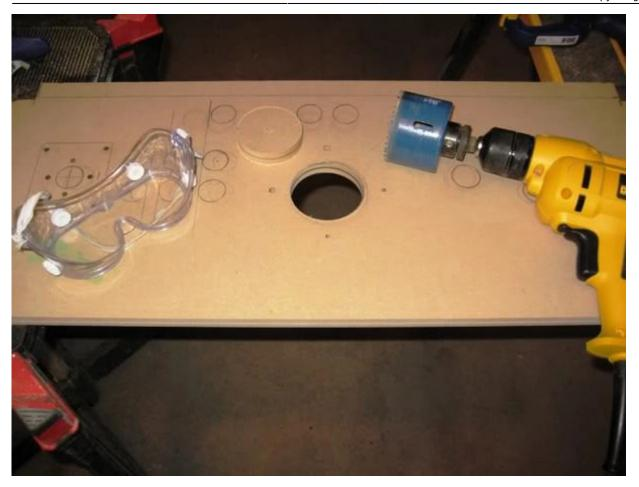
I then drilled the button holes (1 1/8" forstner bit) and joystick/trackball holes (1 1/8" forstner bit). Everything will be top and flush mounted so the laminate will cover all bolts including the trackball. The joysticks will be top mounted using FrancoB's technique as they are JLWs:
