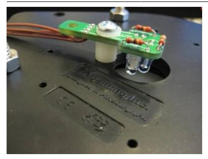
I then connected the Novagems to the buttons. Here is the spare IL translucent green after I drilled it (I ordered replacements from RandyT but will just keep those as spares when they arrive):
