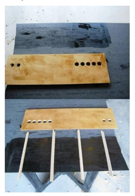
Both the top and bottom of the panel were angle cut to rest flush on the CP and Coin door:
