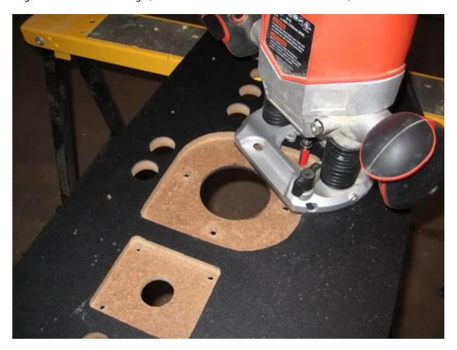
I then route the Trackball recess, note the mod friendly hole at the bottom for RGB lighting (Betson's have these too):
