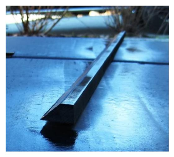
I also used my table saw to cut an angle on the edge that will sit on the angled bezel so it will be flush:
