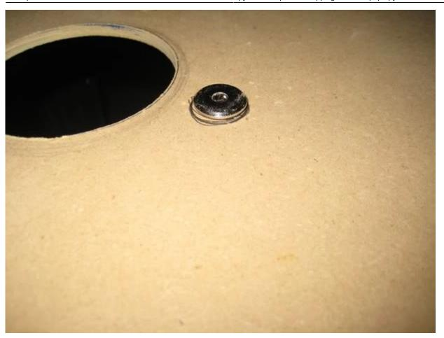
Then routed out 1/16" of MDF for a flush fit. I left a bit of space so that once the CP is ready to get laminated I will glue the bolts in place:
