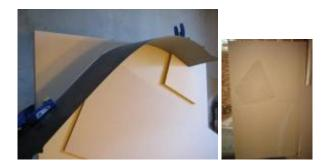
I used a large chunk of leftover rectangular laminate...approx 8" wide by 60" long. You can see this in one of the above pictures. Using clamps I held the back of the curve in place. I would then trace with a pencil along the inner side of the curve. I would start at one end but just a bit ahead of my pencil (maybe 12") I would place a counterweight like wood etc to push the laminate against the clamps from behind, maintaining the curve.
