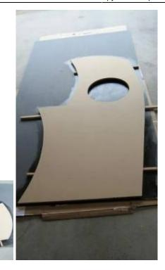
Here is the outside of side 1 fully laminated before and after side hole was trimmed:
