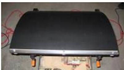
Then I laid it atop one of the side panels to ensure everything including the curves lined up. This turned out perfect and rides just a few mm shy of where the T Molding will run on the side panels along the top and back:
