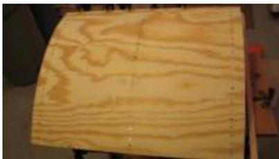
And a closeup of the screws. You can see in this shot they are all countersunk which ensured no contact with the laminate:
