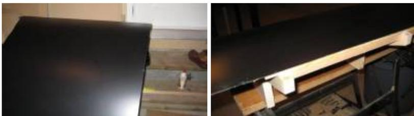
Then I gave it a good trim with the router and as mentioned my bottom bearing trim bit which rode the bottom 1/8" of the 1/4" plywood. This was quick and effortless. Here you can see a shot from the top of the front where the marquee retainer is bolted in. The Retainer and Bolts will be green. I will also laminate the top portion just above the retainer so you won't see the plywood:
