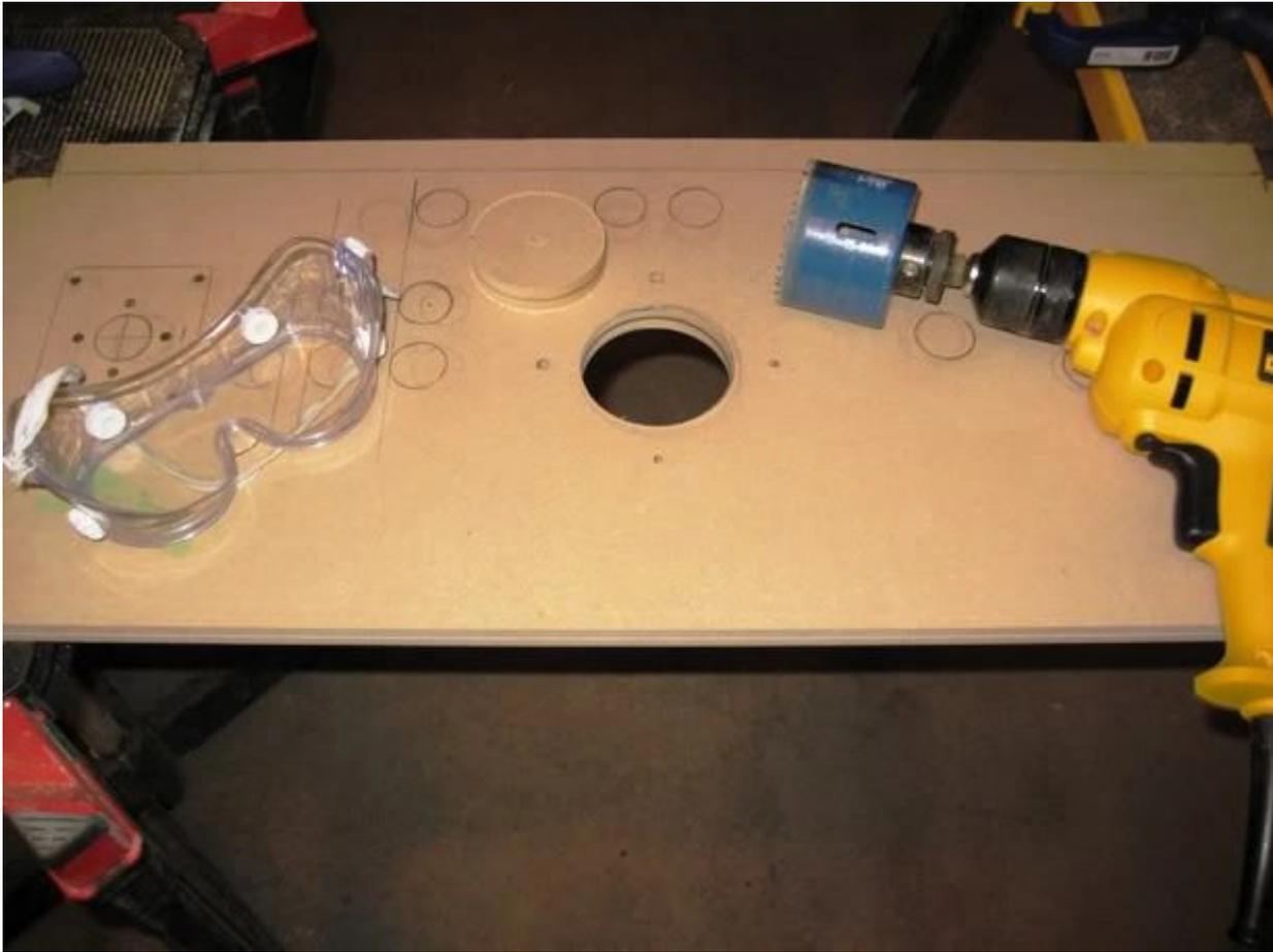
I then drilled the button holes (1 1/8" forstner bit) and joystick/trackball holes (1 1/8" forstner bit). Everything will be top and flush mounted so the laminate will cover all bolts including the trackball. The joysticks will be top mounted using FrancoB's technique as they are JLWs:
