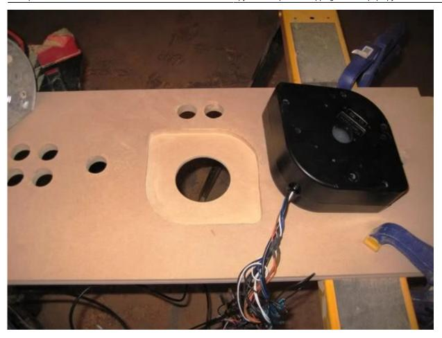
Next up is drilling the bolt holes to hold the trackball. Rather than eyeballing I just drill through the holes with the trackball in place:
