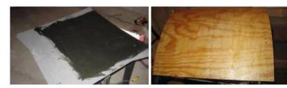
Then I prayed to the 4 winds, Crom and any other deity that would listen and applied the laminate to the top. There isn't a 2nd chance on setting and thankfully it lined up perfectly along the front where I wanted about 2mm of overhang:
