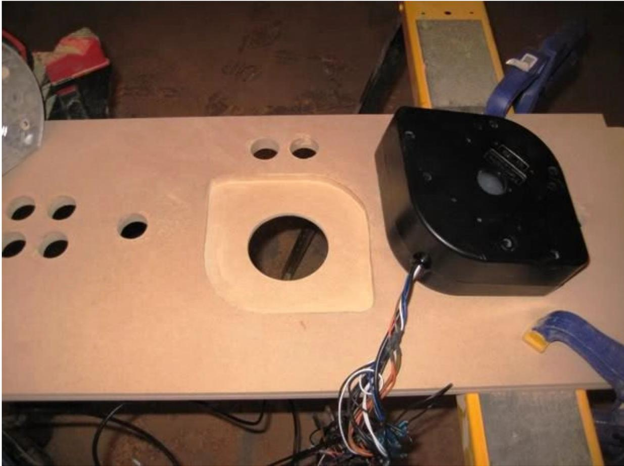
Next up is drilling the bolt holes to hold the trackball. Rather than eyeballing I just drill through the holes with the trackball in place:
