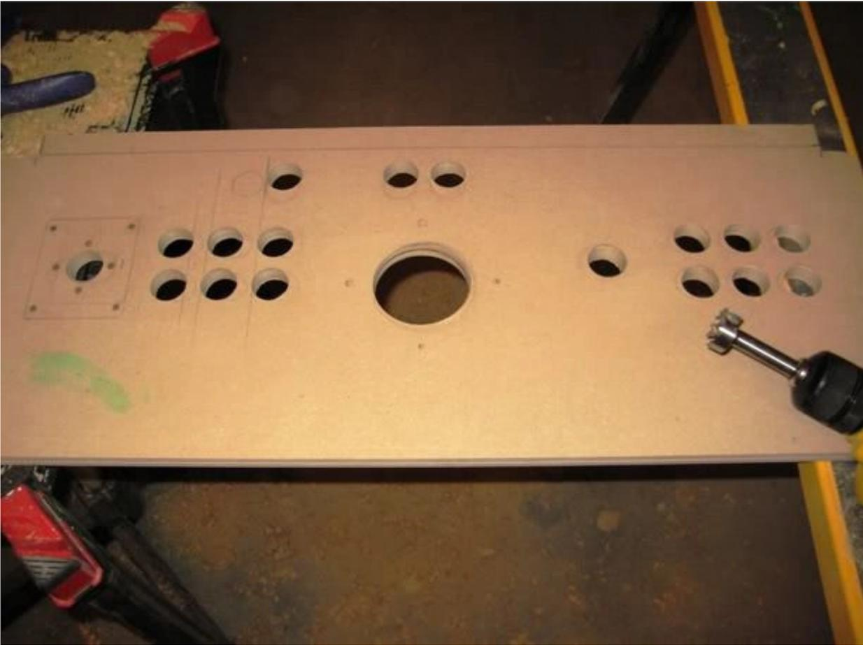
Next step was to place the trackball through the hole and line it up for tracing the part that will get recess routed:
