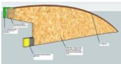
The diagram shows the bottom of the ribs being flat and extended to the bottom of the curve in a straight line. In reality I will make only a 5" portion flat...the rest will curve along approximately 3" from the top. I have tested the plywood and it curves perfectly (and as Ond mentioned...easily) along the top. Over the next few days I will glue this on once I have everything lined up. Overtop of the plywood will sit the laminate.
