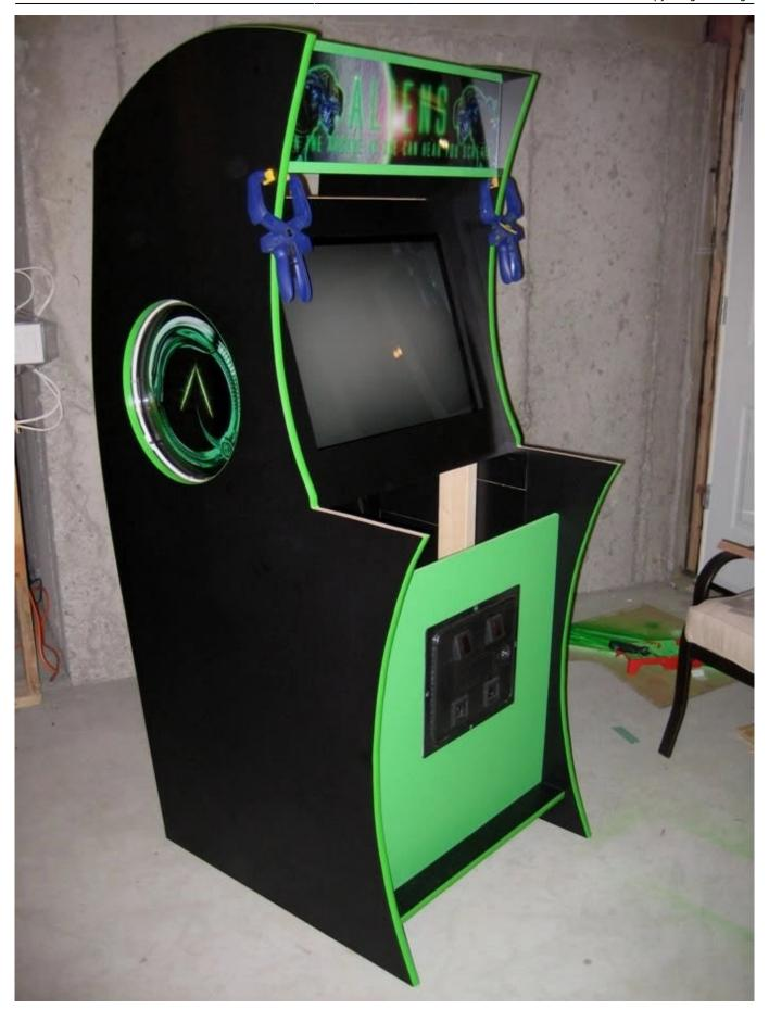
I use Lepage's blue contact cement from Home Depot to laminate the cabinet...it looks like the alien slop but spreads on super easy with a disposable paint brush. It also dries quickly but not too quickly...in other words it gives you enough time to apply glue on both sides before joining (15 to 20 mins).
