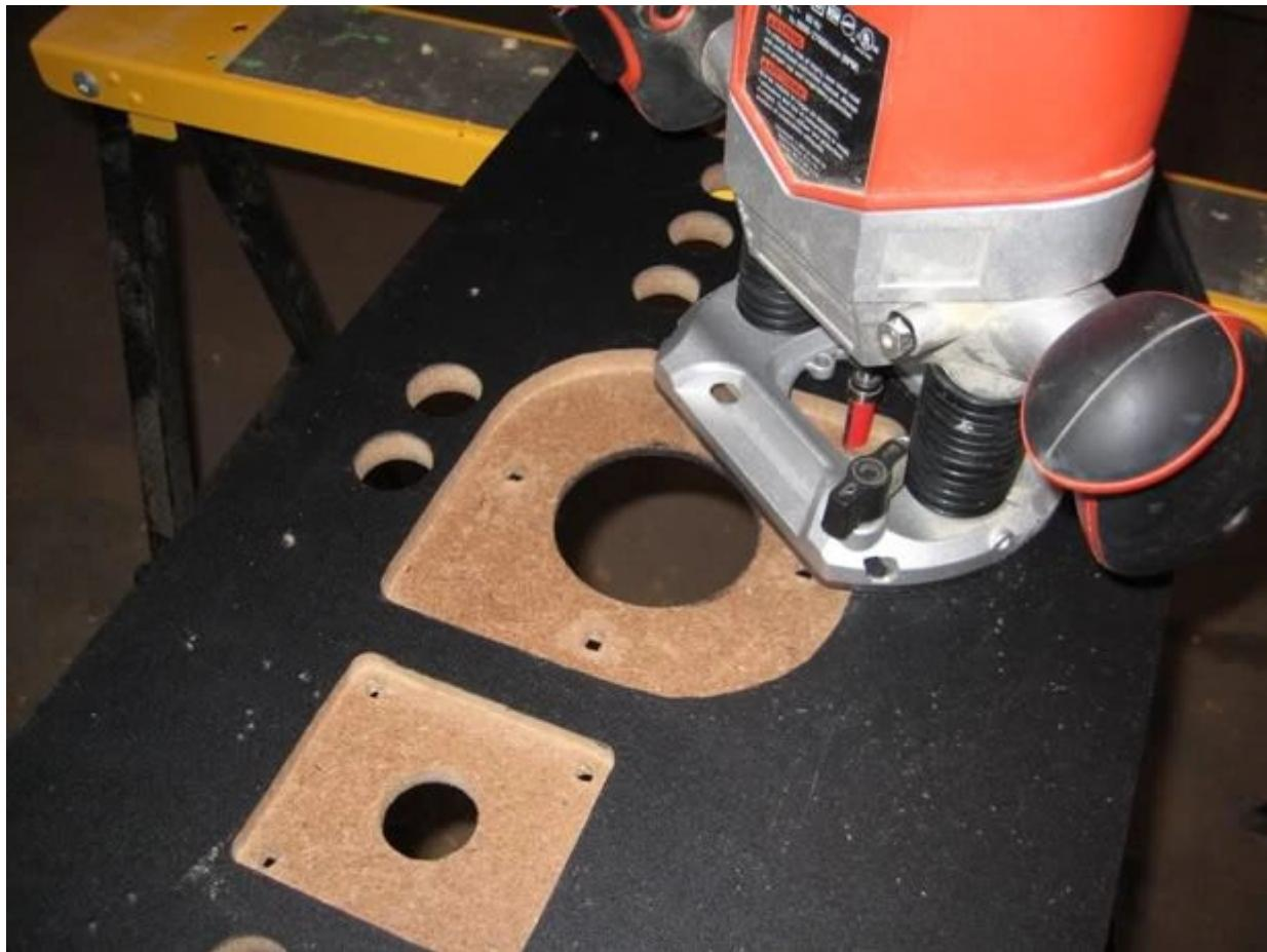
I then route the Trackball recess, note the mod friendly hole at the bottom for RGB lighting (Betson's have these too):
