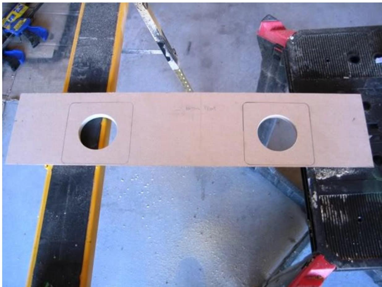
Next step was to laminate the bottom of the shelf that will face the CP. I glued both sides. You may have seen it earlier in my thread or on other threads but a great way to line up your laminate and wood is to use small dowels. I used 1/4" offcuts.
