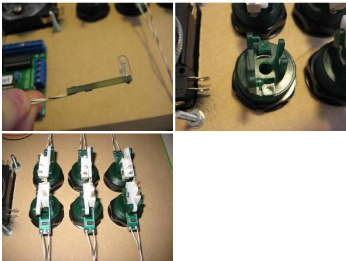
Here is the wiring complete for the LED Wiz...the mini rats nest on the top left will be organized further...getting tired! You can see to the right of the nest a euro terminal block that is feeding the 5 volts for the Lighting. The 5v runs to a hacked molex plug which will hang beneath the CP.
