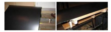
Then I gave it a good trim with the router and as mentioned my bottom bearing trim bit which rode the bottom 1/8" of the 1/4" plywood. This was quick and effortless. Here you can see a shot from the top of the front where the marquee retainer is bolted in. The Retainer and Bolts will be green. I will also laminate the top portion just above the retainer so you won't see the plywood:
