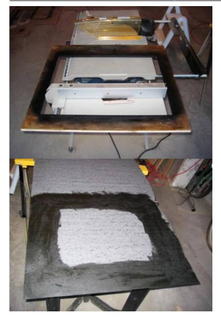
Once the laminate was trimmed, I taped it up and added another 2 coatings of black to the inner portion of the bezel.
