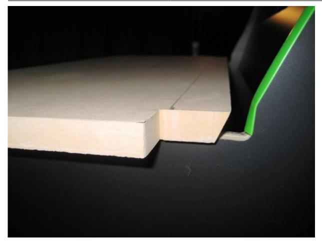
Note there is just enough space between the edge of the cab and the CP for the black T molding of the CP to fit.
