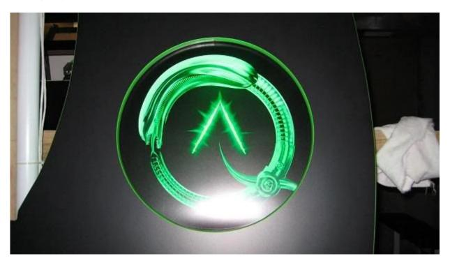
And a few lit pictures...I just dangled the light from behind...no diffusion yet which I will do with a back layer of frosted plexi (art will be sandwiched...reg plexi...art...frosted...cathodes...foil and backing). The pictures don't capture how great this looks even with it not being diffused. For one the art is clear and not shadowy looking and the black surrounding and in between the graphic doesn't have a green smear:
