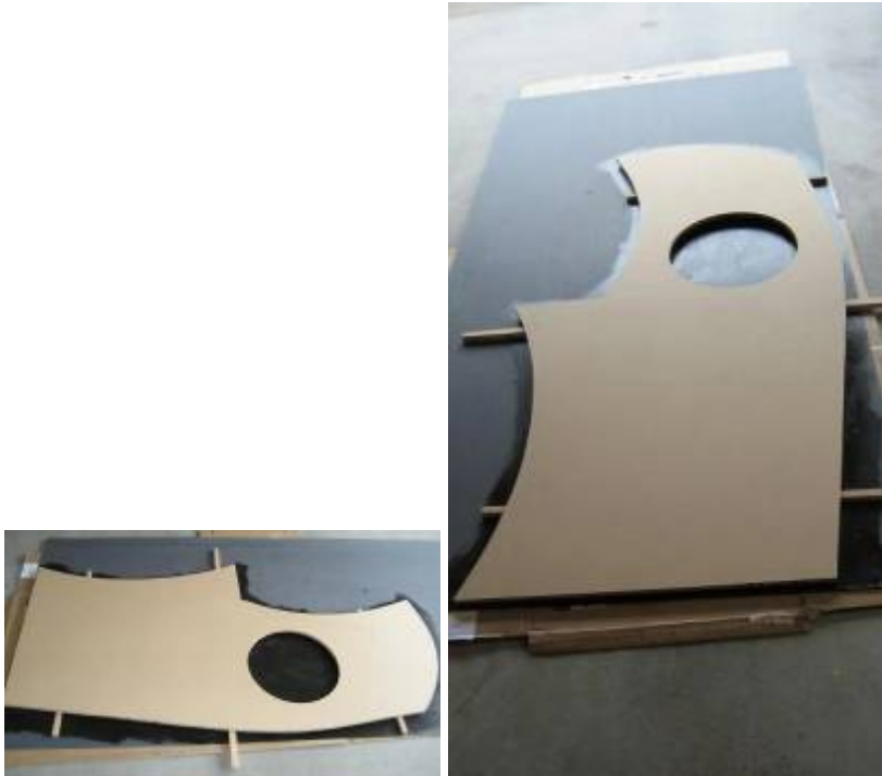
Here is the outside of side 1 fully laminated before and after side hole was trimmed:
