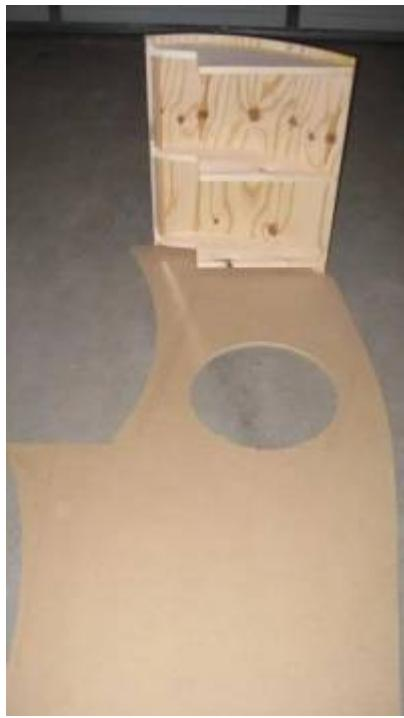
Notice the gap between the side of the cab and the outer rib in the picture below. That is where the a rib will be attached to the side of the cab and the top piece will sit atop and bolt into.
