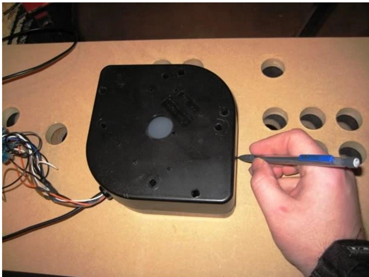
After tracing the mount I went back to my X Gaming CP to set the depth of my router. Both CP's are 5/8". I prefer this size for a CP when using laminate as it's easy have the T molding cover flush the edge of the laminate. Using 5/8" CP I will route the Trackball recess to 1/4" of MDF left:
