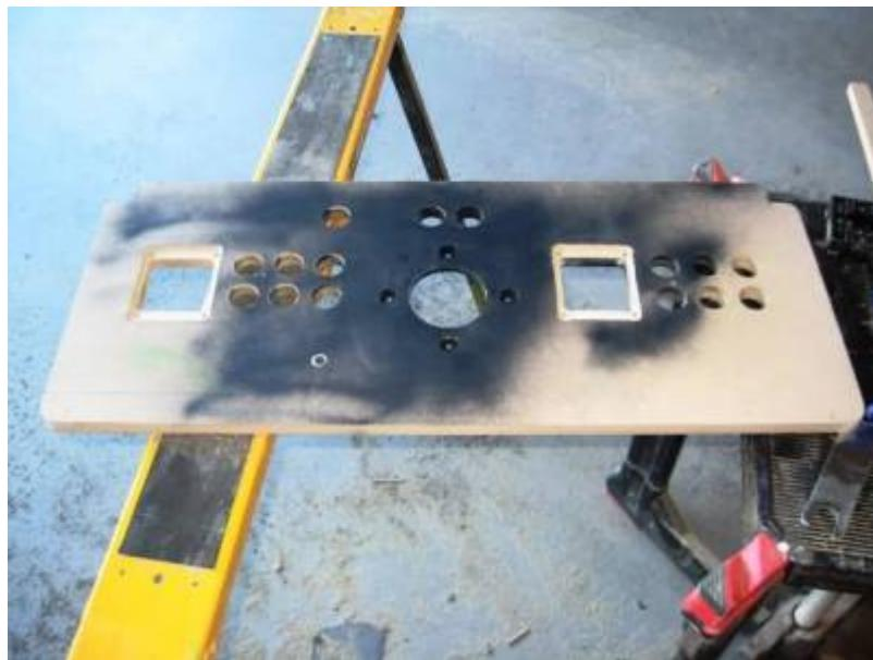
Perfectly flush. I used 6-32 flat head bolts which barely add any height to the profile...less than 1mm:
