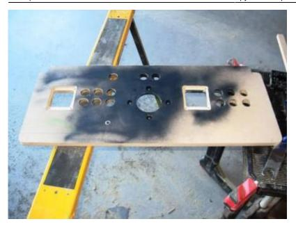
Perfectly flush. I used 6-32 flat head bolts which barely add any height to the profile...less than 1mm:
