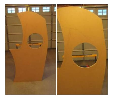
I cut a slot into the center of the hole as I will be running the T-Molding around the hole like I have seen on a few other cabs. I think it will look pretty good when done with the green neon light and artwork and T Molding as a trim:
