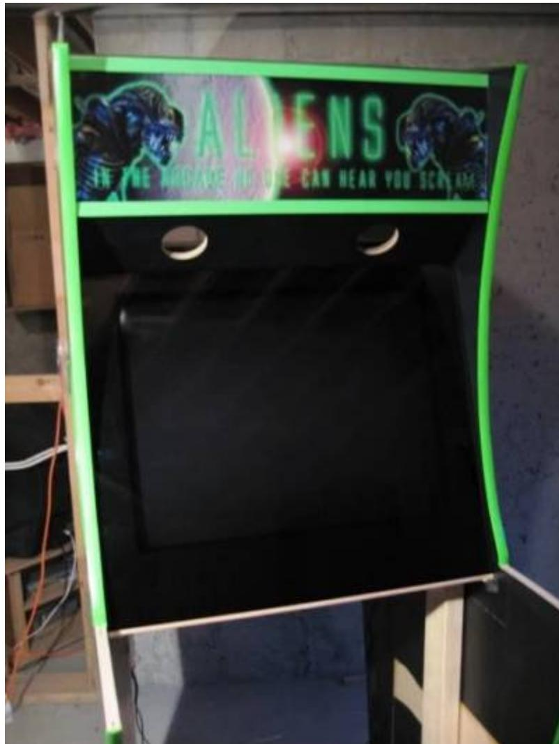
I then realized my CP was cut to not take into account plexi over the bezel...oops...no big deal. I throw it on the table saw and do another 1/4" angle cut so it rests on the plexi flush. I also cut the T mold slot and rounded the edges. Lastly, I used my X arcade to template sketch the buttons (6 each player), trackball, p1/p2 and Spinner (to left of p1/p2):
