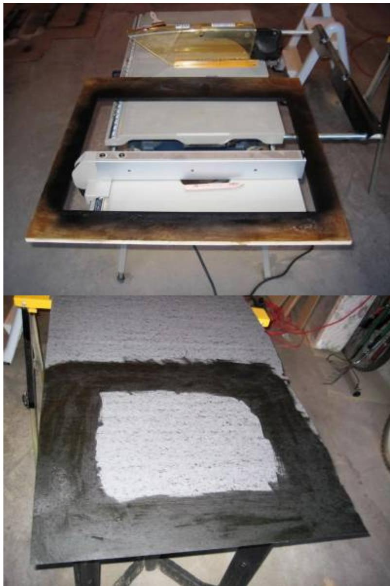
Once the laminate was trimmed, I taped it up and added another 2 coatings of black to the inner portion of the bezel.
