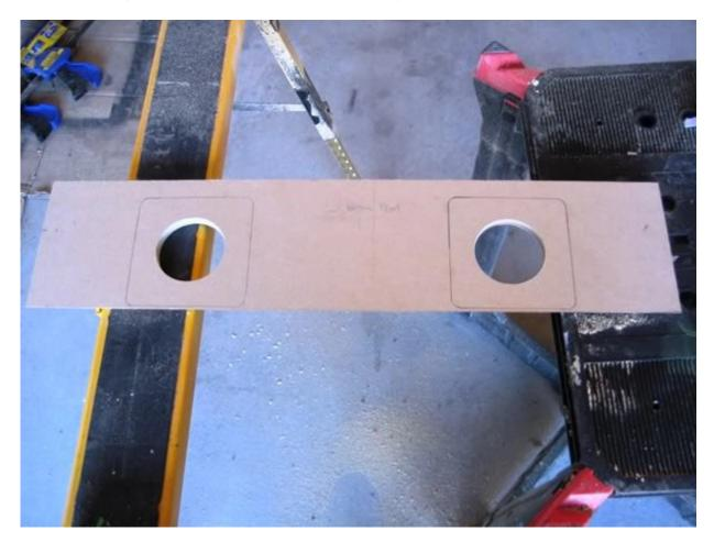
Next step was to laminate the bottom of the shelf that will face the CP. I glued both sides. You may have seen it earlier in my thread or on other threads but a great way to line up your laminate and wood is to use small dowels. I used 1/4" offcuts.
