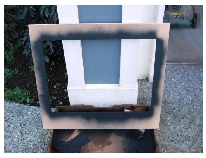
Once the 3 coatings had dried I traced out the bezel on the back of the laminate and then applied glue to both the mdf and the underside of the laminate. I let it dry for about 20 minutes before joining and trimming the laminate.
