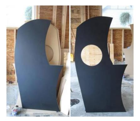
I then laminated the inside which you can see is a patchwork of odds and ends. I put as much towards the center as I could because I will be mounting strips and don't want parts of the strip on laminate and part off:
