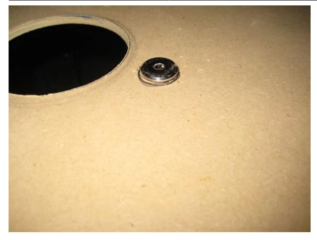
Then routed out 1/16" of MDF for a flush fit. I left a bit of space so that once the CP is ready to get laminated I will glue the bolts in place:
