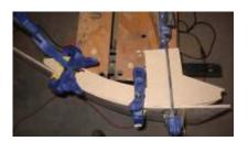
Each side of the cab will have one of the ribs (made of pine or harder wood) connected to it with threaded inserts. The main stress will be downward and the vertical inserts will take the load off the few horizontal ones I use (like these). You can also see on this picture the idea behind the curved skelton. It will continue in a 2nd piece that will curve along the back to the bottom so that what I end up with is a nice curve outlining the cab...no squares here.
