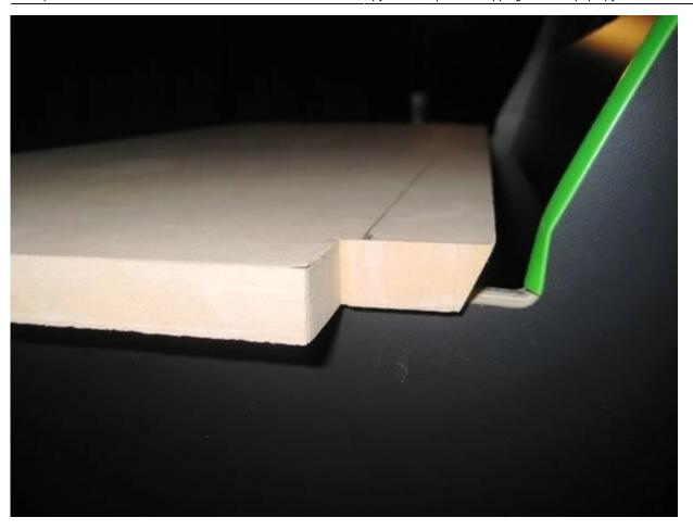
Note there is just enough space between the edge of the cab and the CP for the black T molding of the CP to fit.
