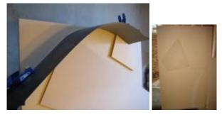
I used a large chunk of leftover rectangular laminate...approx 8" wide by 60" long. You can see this in one of the above pictures. Using clamps I held the back of the curve in place. I would then trace with a pencil along the inner side of the curve. I would start at one end but just a bit ahead of my pencil (maybe 12") I would place a counterweight like wood etc to push the laminate against the clamps from behind, maintaining the curve.
